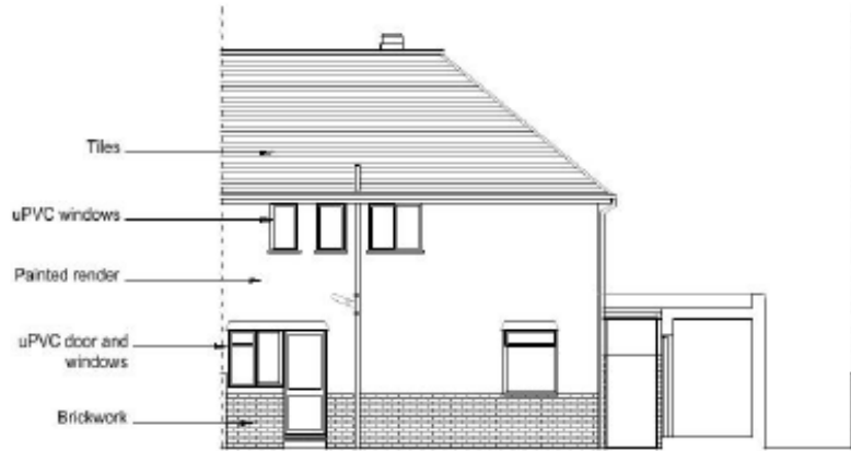
Existing Rear Elevation 1:100
